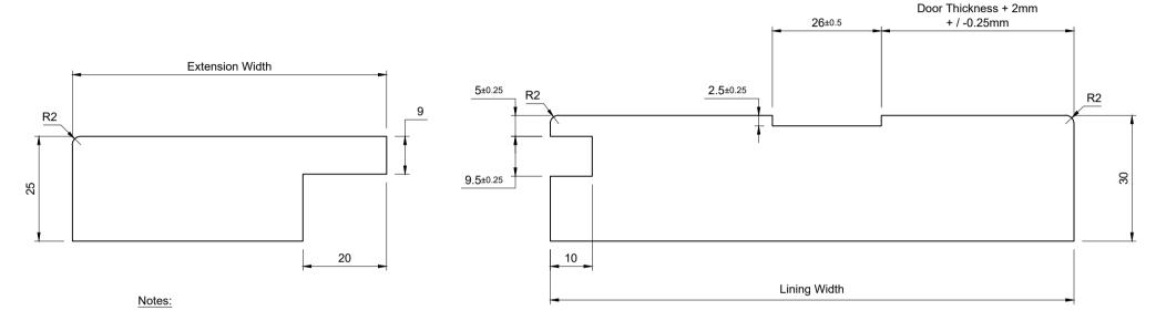
Extension Head Length = Lining Head Length Extension Head Rebate = Extension Head Length - 50mm Extension Head Rebate Depth = 11mm Extension Jamb Length = Lining Jamb Length - 2mm
